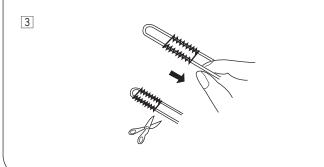
3 Pull the loose ends of the filler cord to tighten it.
