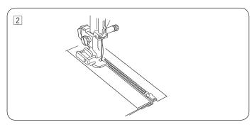
2 Attach the zipper foot with the pin on the right. Sew through all the layers from the end of the zipper opening, guiding the zipper teeth along the edge of the foot.
