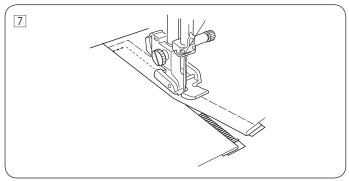
7 Open the zipper, then lower the foot and stitch the remainder of the seam. After finished sewing, remove the basting stitches on the upper fabric.
