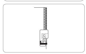
This stitch can be used for sewing fabrics that tend to fray extensively such as linens and gabardines. Two rows of zigzag stitches are simultaneously sewn over the edge to ensure that your seams will not ravel. Adjust the thread tension so both the needle and bobbin threads meet at the edge of the fabric.
