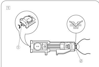
Use the same procedure as the square buttonhole procedure. Set the stitch width to match the thickness of the cord used. With the buttonhole foot raised, hook the filler cord on the spur ① at the back of the buttonhole foot.
