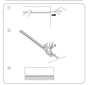
Fringing adds a special touch on table linens and shawls. Choose a firm, woven fabric like linen where threads can be removed easily.
