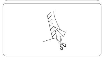
Place your fabric to allow a 1.5 cm seam. Trim excess close to the stitching. Be careful not to cut the stitches.
