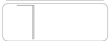
For seaming garments, zipper application and more. Pattern 03 is used for seaming fine fabrics.
