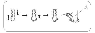
The sewing procedure is the same as the square buttonhole. Use the seam ripper and an eyelet punch 4 to open the buttonhole.
